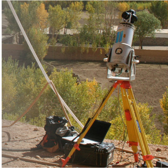
Fig. 5 Laser Scan System Riegl LMS 420i with on-top mounted digital camera (acdc 2006/Irmengard Mayer)
